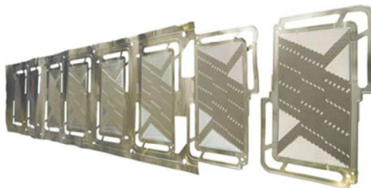
Figure 2: Metal strip of the NM5 bipolar plate produced with a progressive die set.
